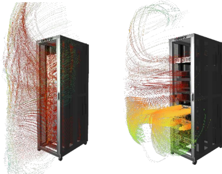
Figure 6: Cabinet-level exhaust airflow pattern for a design cabinet (on the right) containing the same equipment with an evenly distributed load and an operational cabinet (on the left) with differing IT and power densities
